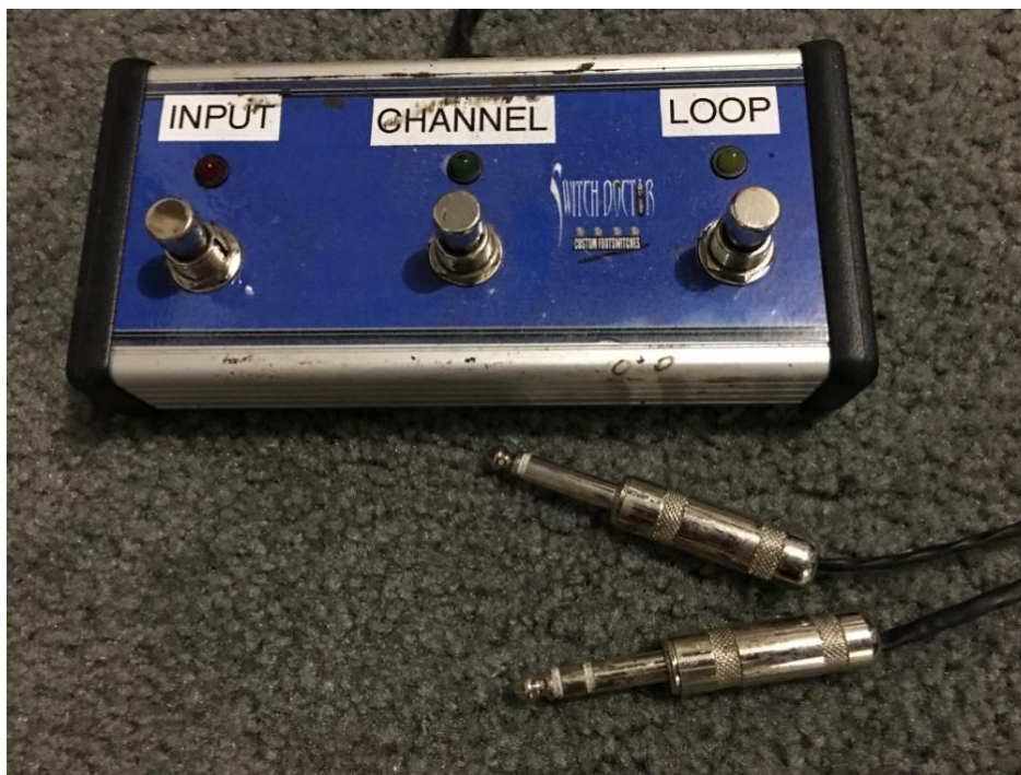
Custom three button footswitch wired for a stereo plug for the loop and channel functions, with a mono plug for the input function
