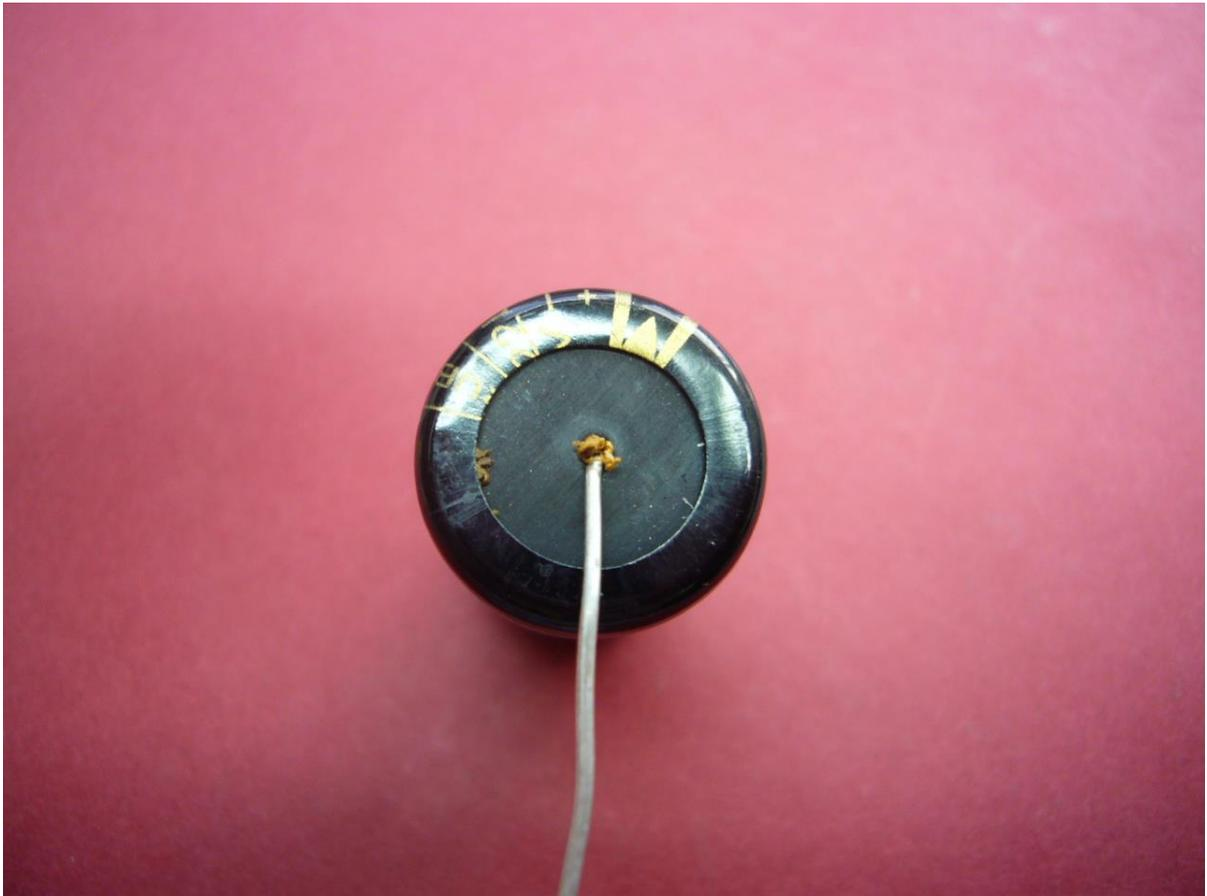
*The filter caps are easy to replace. Cut the cable tie and the leads on the cap. There is also some glue between the board and the component. Gently break the cap out:*
