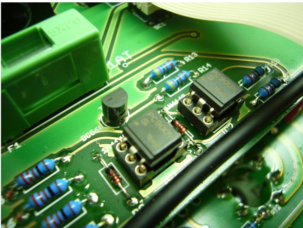
If you do not have a special tool to remove the old controller chip, alternate prying each end out bit by bit with a small screw driver until the chip comes free:
