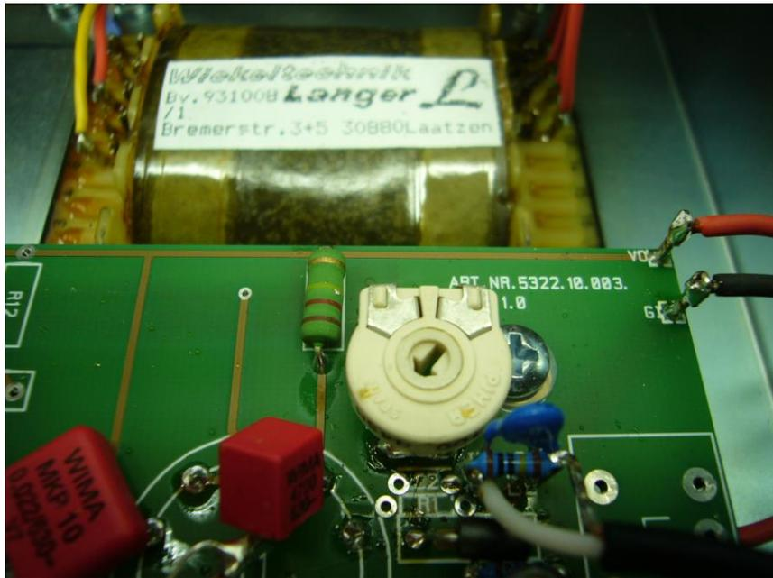
*Remove the trim pot with a solder iron and refresh the 4 solder pads on the PCB:*
