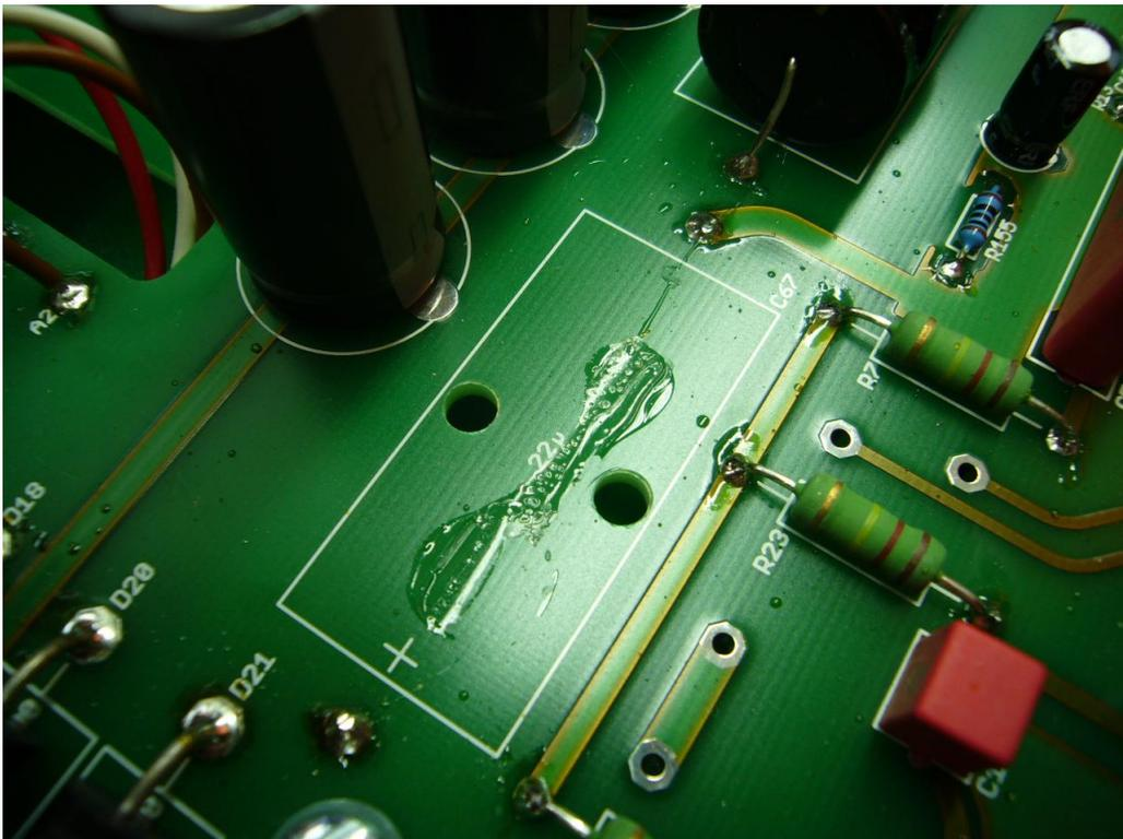
*25 Replace the cap with a proper substitute checking for correct polarity orientation and glue it on the board to avoid movement.*
