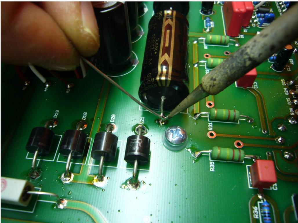
*To avoid further damage to the caps we recommend to replace one resistor in the power supply. This a resistor with 2,2k ohm / 9 watt as in the picture below:*
