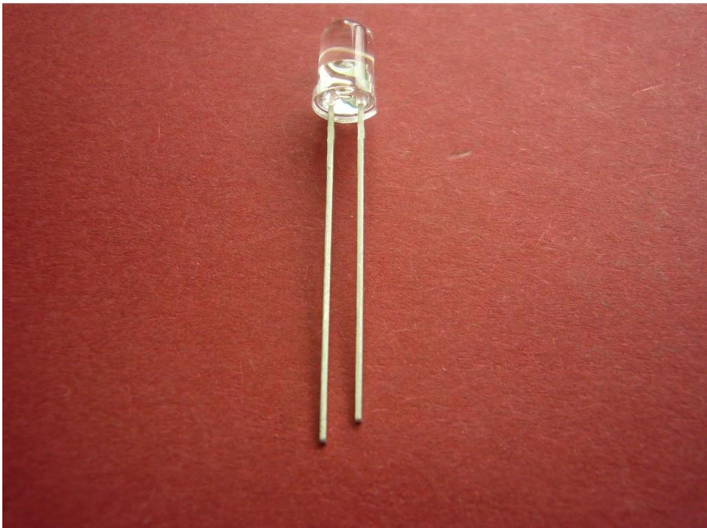
*Shorten the pins on the LED a bit for good fit, and solder the LED to the board. Bend the leads to get the LED through the*
