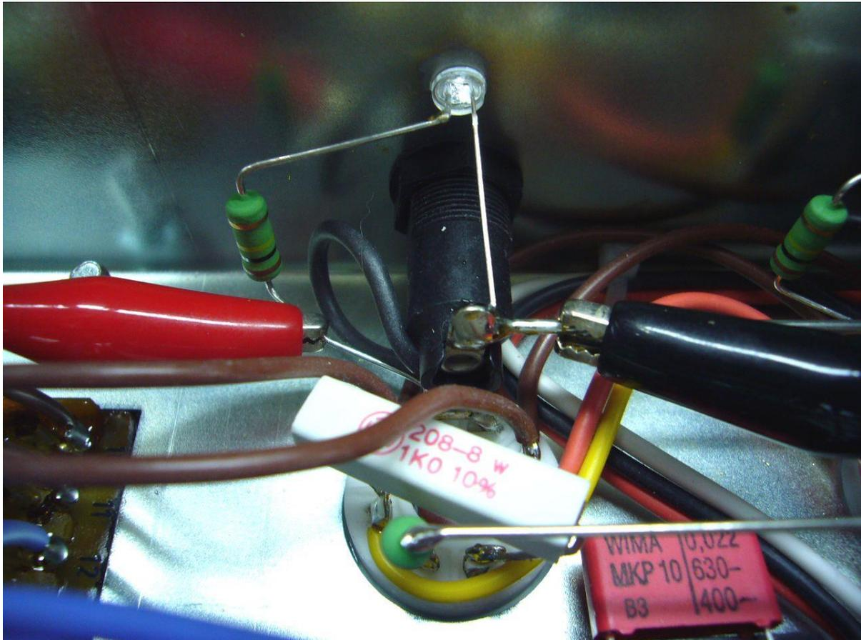
*Adjust the bias trim pot with a small screwdriver to approximately 35 milliamps on the multi-meter:*
