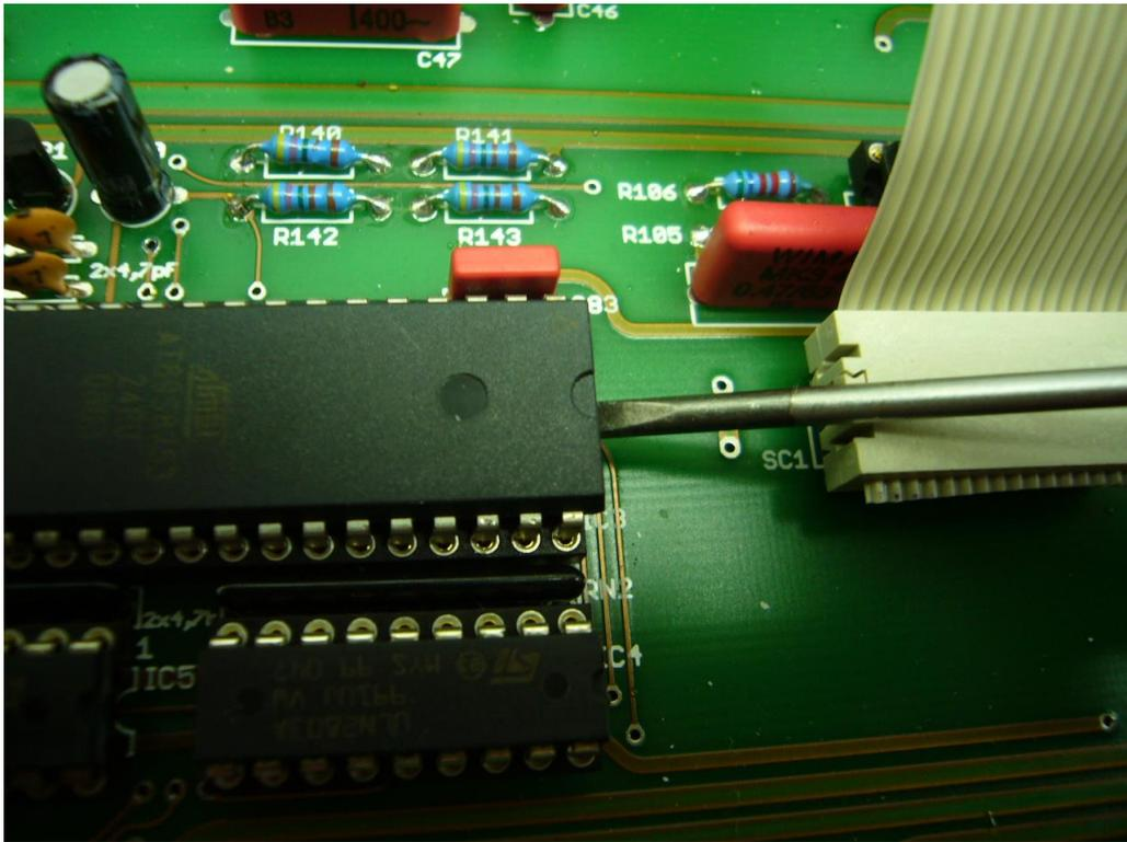
*Check for orientation (half circle tab), and set the new chip. Lastly push the unit snug in the socket.*
