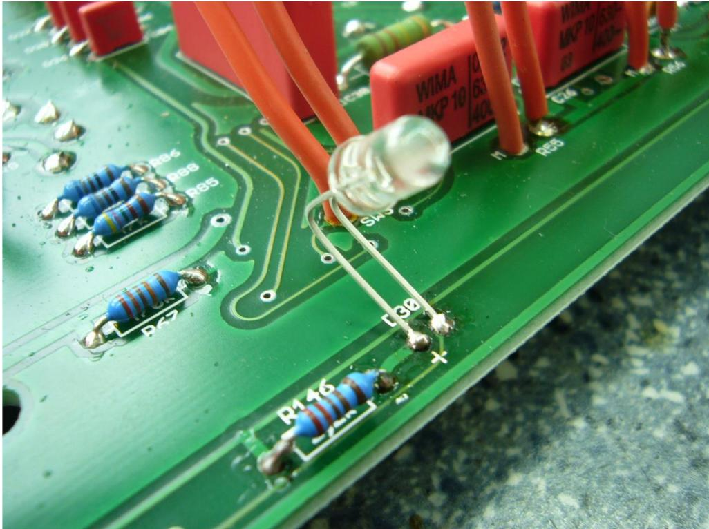
*To avoid further damage to all LED's, we recommend that the pre-resistors are replaced. These resistors are located close to*
