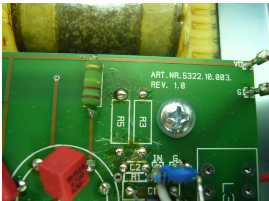
*Now solder the 47 ohm resistor and the 100 ohm resistor in.
